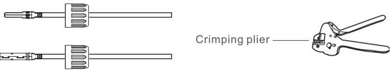
▲ Figure 4.10 Crimp the contact pin to the wire
