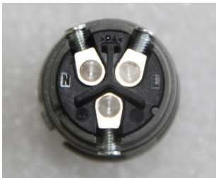
▲ Figure 4.13 AC Grid Terminal Connector Inside
